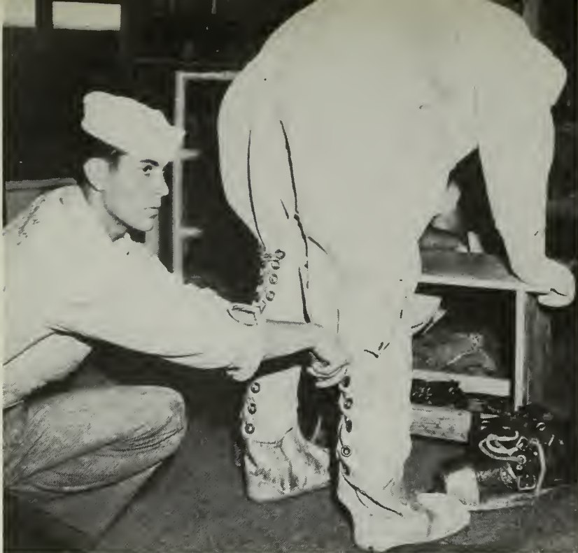
BATTEN DOWN —Legs of diver's suit are laced up the back to keep air out. Air in legs would cause diver to take a horizontal instead of vertical position.
